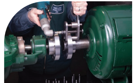
Removal of bushing using tool and angle ratchet wrench
