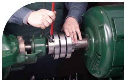
Installation of pins using ratchet wrench
