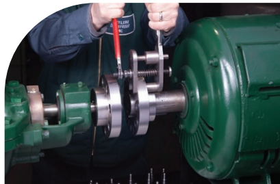
Removal of bushings using tool and ratchet wrench
