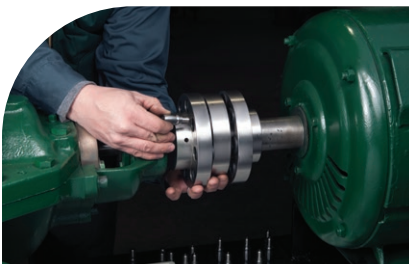
Raising of ring and engaging all pins from both sides by hand (thread locker already applied)
