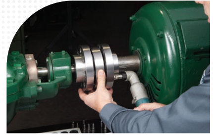
Removal of pins with cordless angle ratchet wrench
